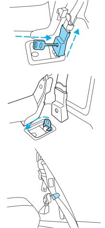
3. Use the black plastic clip (located just above the detachable anchor) to stow the loose seat belt.
